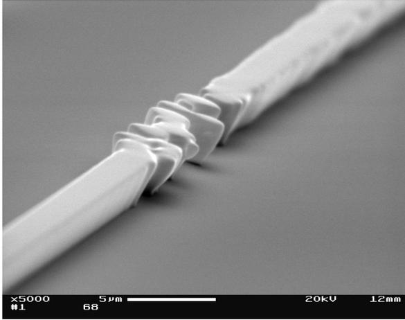
Figure 4.9: High dark erosion as a result of a poor softbaking at 100 °C for 45 s (AZ nLOF 2070 5:1 PGMEA resist on Si) <sup>a</sup>
