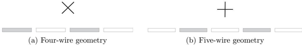
Figure 1.6: Possible configurations for surface-electrode trap. Modified from (14)
