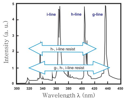
Figure 2.1: Mercury lamp spectrum. Taken from (25)
