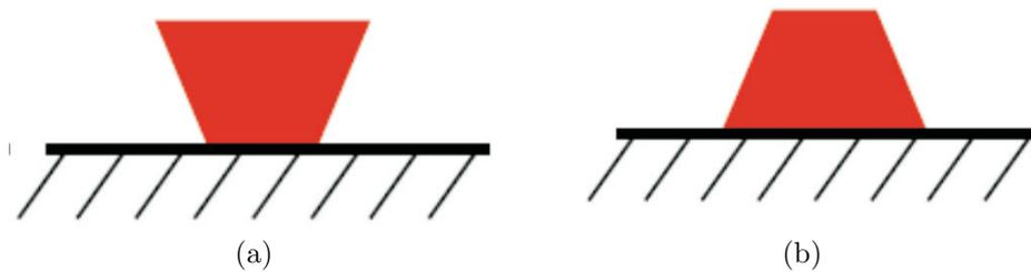
Figure 2.2: Negative and positive resist profiles. Taken from (26)
