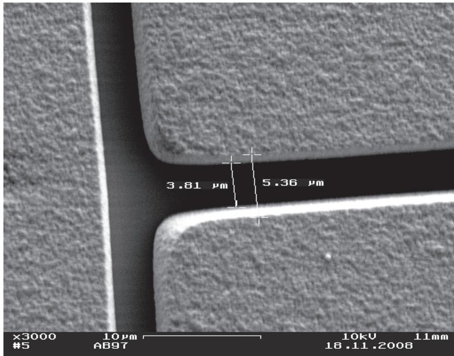
Figure 5.5: SEM image showing the undercut profile achieved in Chip 5. The distance measured at the bottom corresponds to  $3.8 \mu\text{m}$  and on top to  $5.3 \mu\text{m}$ . From image it also is visible that the sidewalls of Au plated electrodes are smoother when compared to top surface. This smooth sidewalls enhance the expected breakdown voltages value.
