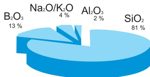
Figure 4.1: Chemical Composition of BOROFLOAT<sup>®</sup> 33. Taken from (28)
