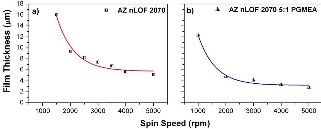
Figure 4.8: To make the spin coating process more reproducible I decided to coat Si wafer and measure the film thickness as a function of spin speed of a) non-diluted and b) diluted AZ<sup>®</sup> nLOF 2070 5:1 PGMEA resist
