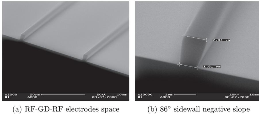
Figure 4.12: The resist mask shown in these pictures was achieved with a development time for 110 s in AZ<sup>®</sup> 826 MIF, previously exposed during  $45.90 \text{ mJ/cm}^2$  with a soft-bake at  $100^\circ$  for 60 s and a post-exposure bake at  $120^\circ$  for 60 s.
