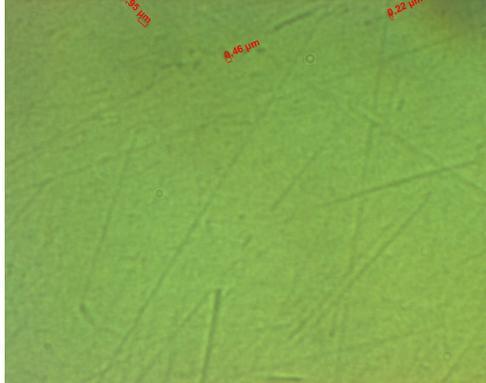
Figure 4.6: Thriving results achieved by employing the spin coater method. There is no considerable dirt on glass surface after this process. Although, some dirt particles below  $1\ \mu\text{m}$  are observed, which might not strongly affect the resist patterned structures. (x100)
