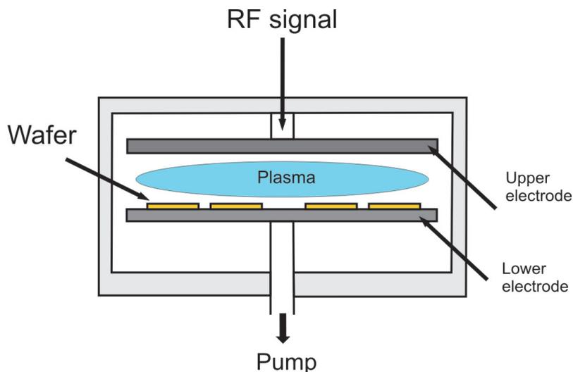
Figure 2.9: Scheme of a RIEO<sub>2</sub> reactor
