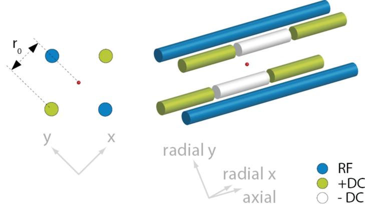
Figure 1.4: Standard four-rod, linear RF trap. Taken from (22)
