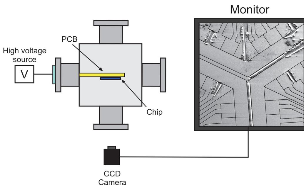
Figure 5.1: Setup for a real-time electrical breakdown test
