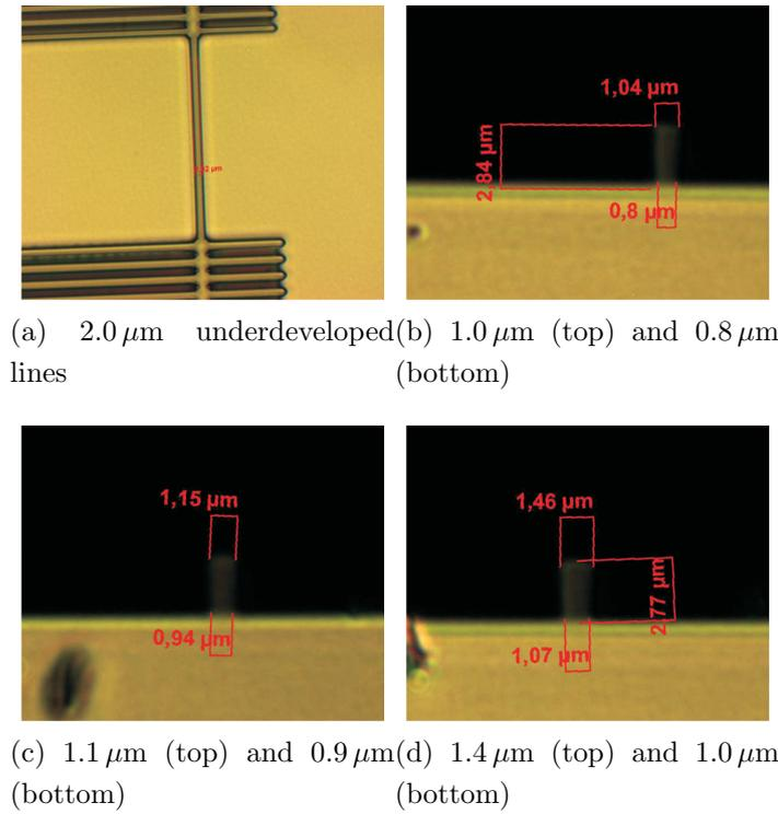
Figure 4.11: After second dose exposure series the exposed 5:1 AZ<sup>®</sup> nLOF 2070 resist, with 17.34 mJ/cm<sup>2</sup>, shows an aspect ratio about 3:1
