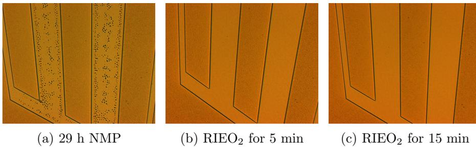
Figure 4.17: Chip 3 is soaked in a 20 mL solution of NMP for 29 h, after which there still exist resist residues. A first cleaning step by employing  $\text{RIEO}_2$  etching means for 5 min presented a visible improvement. A further 10 min by using  $\text{RIEO}_2$  was carried out an effective resist removal was accomplished.
