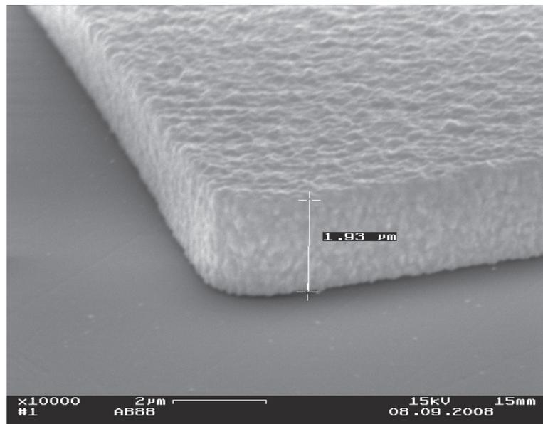
Figure 4.22: For Chip 2 a dilution of gold etchant  $\text{KI}/\text{I}_2 : \text{H}_2\text{O} = 1 \text{ mL} : 2 \text{ mL}$  was selected which showed a visible improvement in surface roughness when we observed it through scanning electron microscopy.
