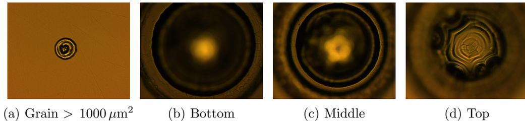
Figure 4.5: A sample which was previously cleaned by means of the two-stage process presented gold grains with an area up to 10000  $\mu\text{m}^2$  after the deposition of 5 nm Cr layer and a successive 50 nm Au layer. A series of defocus technique permits to observe the bottom, middle and top part of the grain. This results strongly suggested to seek for an alternative cleaning method since such large grains visibly prevent any successful lithographic outcomes
