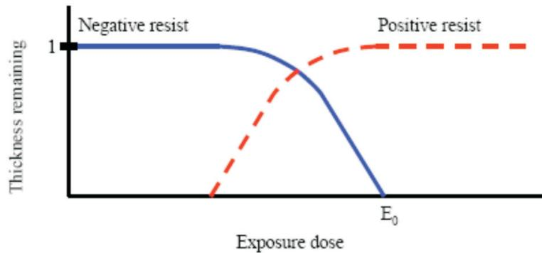
Figure 2.3: Contrast curve of a positive and negative resist plots, the remaining resist thickness as a function of the (logarithmical plotted) exposure dose. For a negative resist,  $E_0$  corresponds the exposure to clear all resist. In the case of a positive resist,  $E_0$  is the lowest required dose to keep resist thickness remaining. Taken from (26)
