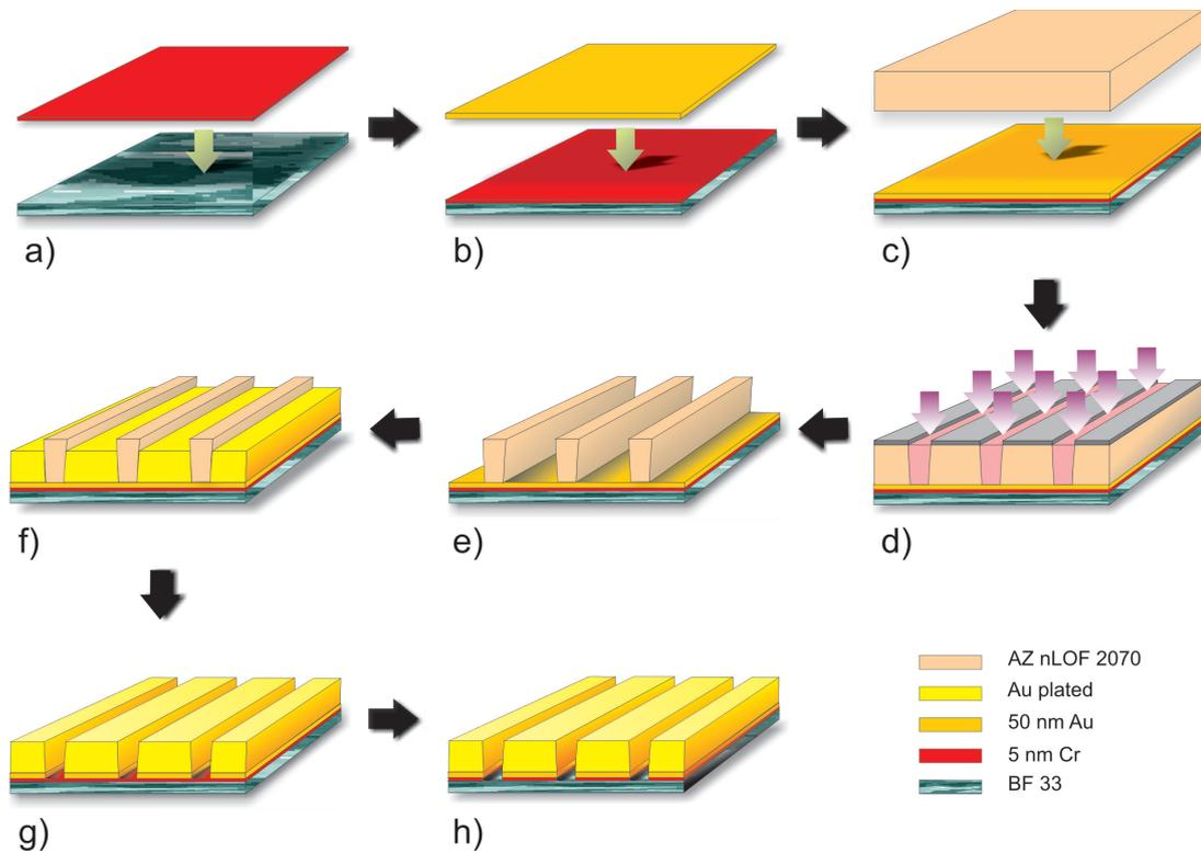
Figure 3.1: A scheme of fabrication process. a) Evaporation of the adhesion Cr layer on BF<sup>®</sup> 33 wafer, b) Evaporation of the starting Au layer on Cr/BF<sup>®</sup> 33, c) Spin coating of AZ nLOF 2070 resist, d) Exposure to UV light, e) Development, f) Electroplating of Au, g) Stripping of resist, h) Wet-etching of Cr and Au layers.
