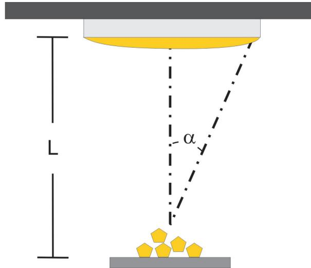
Figure 2.6: Thermal evaporation.
