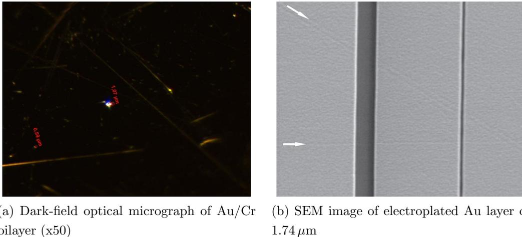
Figure 4.2: The presence of scratches as a result of the polishing process influence the deposited layer roughness in further fabrication steps such as a) Au seed layer and/or b) Au plated electrodes.
