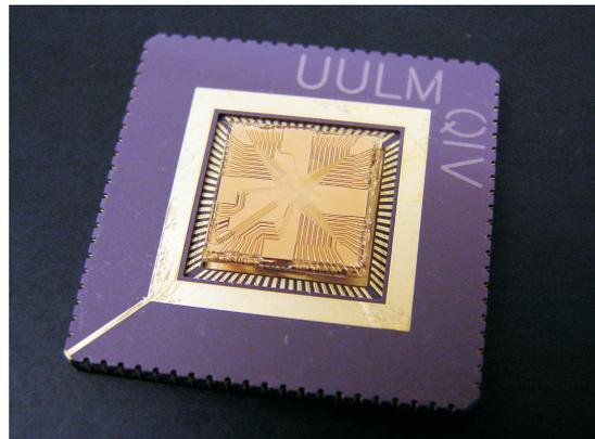
Figure 6.1: Surface-electrode ion trap with an aspect ratio 3:2.
