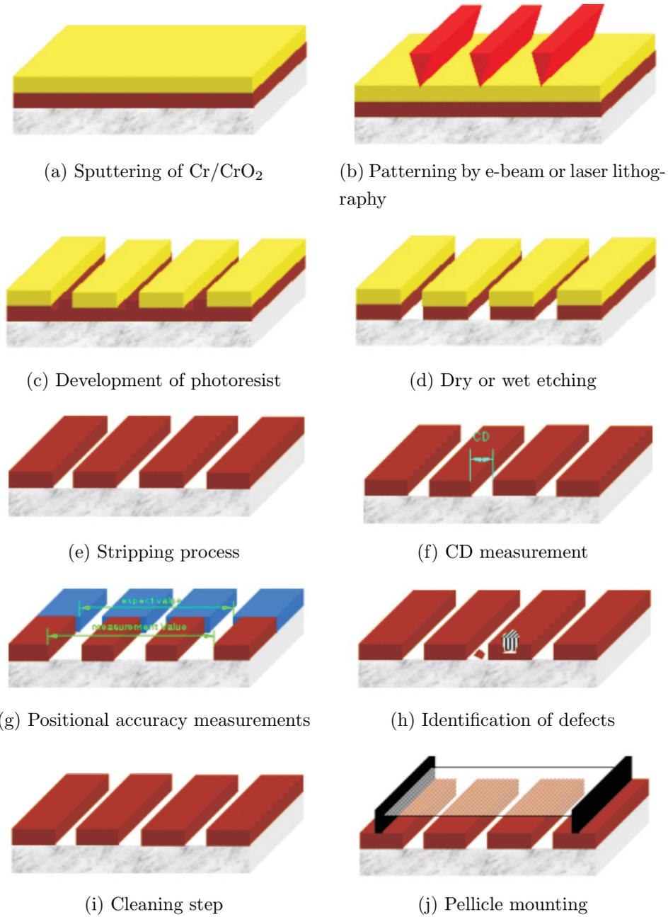
Figure 2.5: Mask fabrication procedure. Taken from (29)
