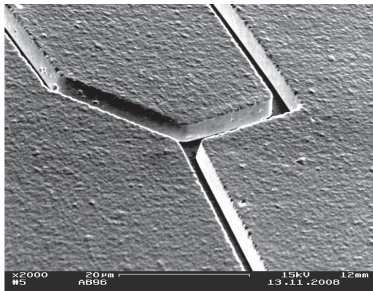
Figure 4.18: This SEM micrograph corresponds to Chip 4 after 2 h in NMP and 20 min in  $\text{RIEO}_2$ . By employing 20 min in an atmosphere of  $\text{O}_2$  it is demonstrated that fully stripping of resist is attained. No resist residue under SEM studies were found. The results by utilizing long time in  $\text{RIEO}_2$  guarantee a successful wet etching of Cr/Au layer.
