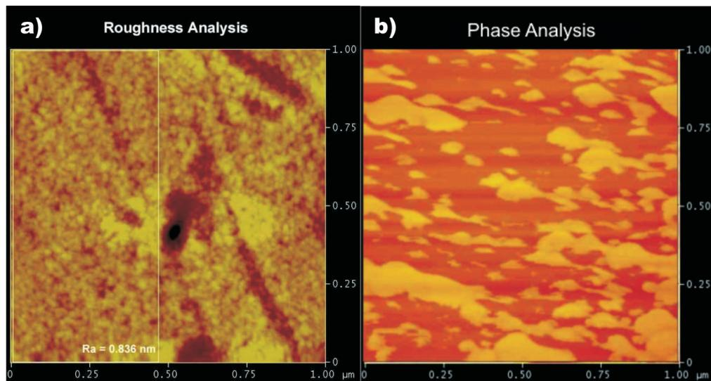
Figure 4.3: AFM topography illustrating a) a) non-cleaned and b) after two-stage process cleaned BOROFLOAT<sup>®</sup> 33 wafer of  $1 \times 1 \mu\text{m}^2$ .
