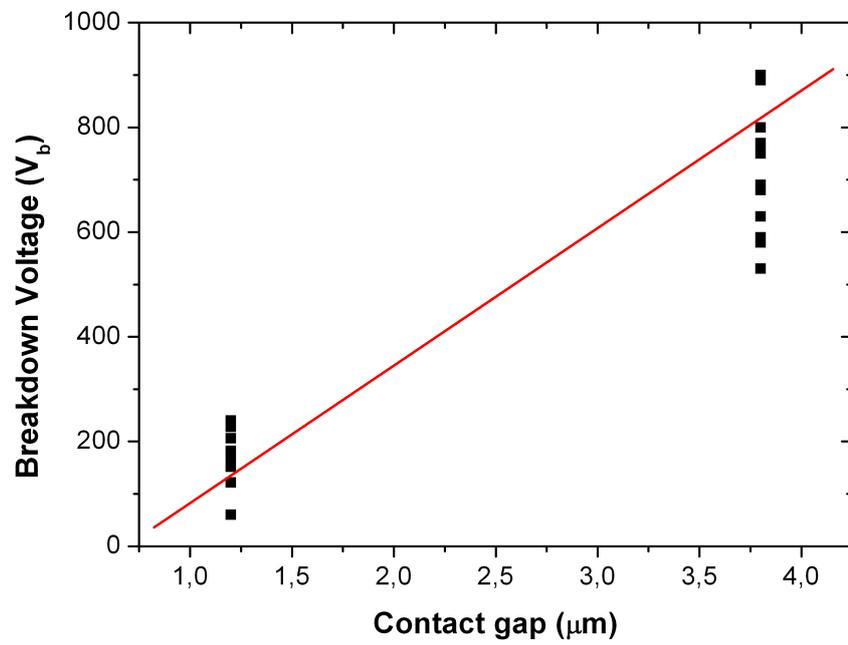
Figure 5.4: It is seen that for a larger gap such as 3.8  $\mu\text{m}$  the breakdown voltage is 720 V.
