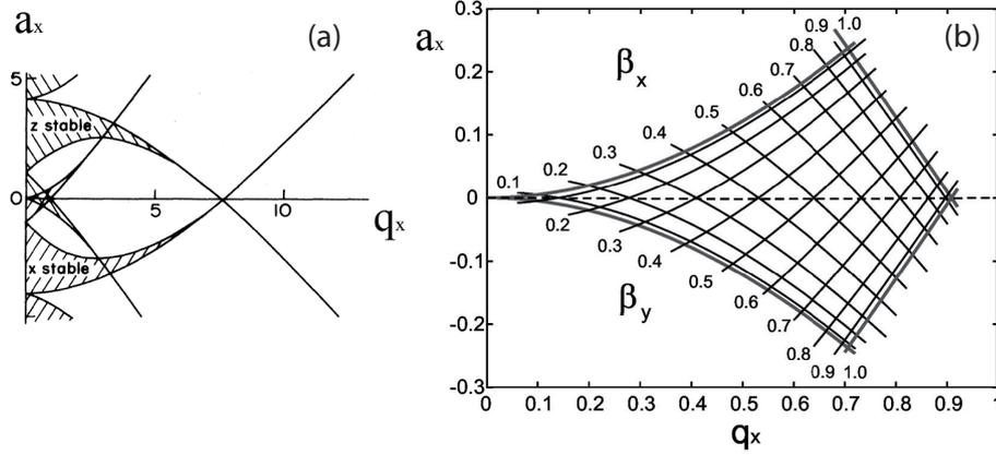
Figure 1.3: Stability domains for a) the ideal 3D Paul trap and b) the lowest stability diagram of a linear RF trap. Taken from (22)
