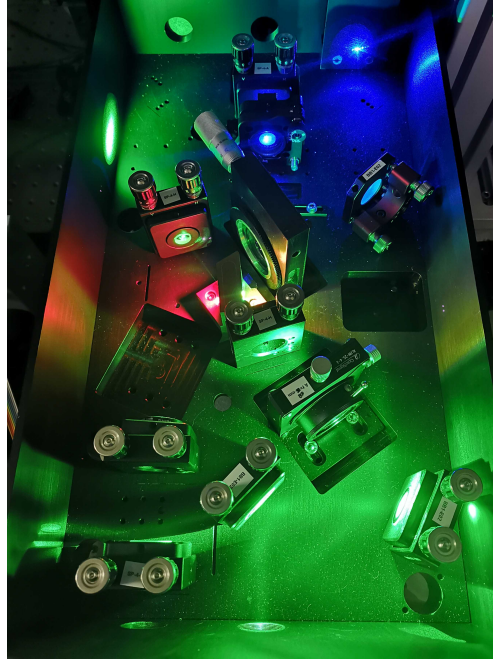
Figure 4.5.: Photograph of the Ti:Sapph cavity. The crystal is visible by its red spontaneous decay signature (670 – 1070 nm). The green pump laser (532 nm) is entering from the bottom of the picture. In the top the frequency doubled blue scattered light (470 nm) from the intra-cavity BBO is visible.
