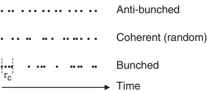
Figure 3.1 Schematic illustration of photon anti-bunching compared to coherent and bunched light. \tau_c is the coherence time of the bunched light.
