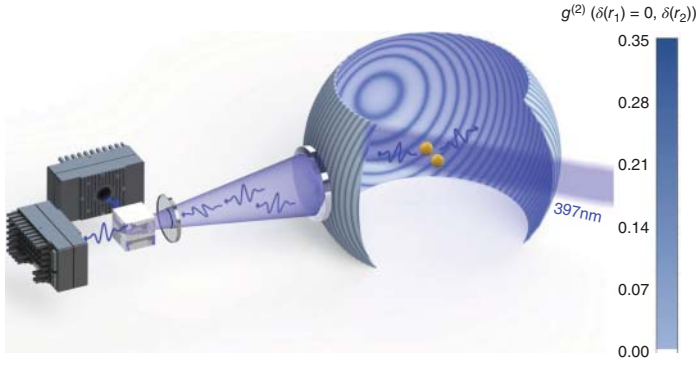
Figure 11.15 To measure g^{(2)}(\mathbf{r}_1, \mathbf{r}_2, \tau) , two ^{40}\text{Ca}^+ ions are trapped and continuously excited on the S_{1/2} - P_{1/2} transition while the scattered light is collected by a lens and, after passing a polarization filter, fed into a Hanbury–Brown and Twiss setup using two MCP cameras. The sphere around the two ions sketches the spatial pattern of g^{(2)}(\mathbf{r}_1, \mathbf{r}_2, \tau = 0) as a function of \mathbf{r}_2 for \delta(\mathbf{r}_1) = 0.34\pi .
