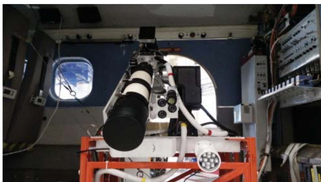
Figure 25.5 The receiver apparatus facing out the port-side door of the NRC Twin Otter research aircraft. Source: Pugh et al. [21]/with permission of IOP Publishing.
